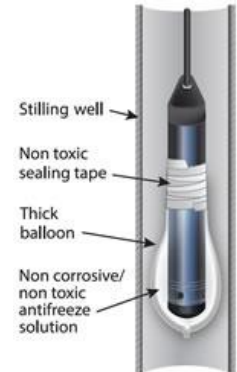
Figure 1: Winterizing the Levellogger
